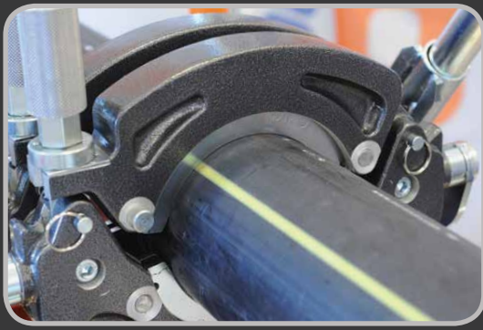
Self-centering and precise jaws/clamps
