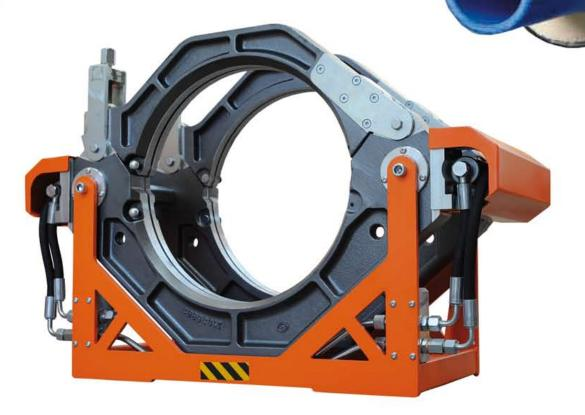
COMPACT 355 L is a worksite machine for pre-insulated pipes in PE, HDPE, PP, from Ø 4" IPS + 14" IPS (125 ÷ 355 mm). Its small dimensions allow it to operate easily inside a dig, plus:
